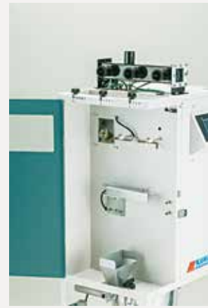
Removable hopper for main material and M/B
